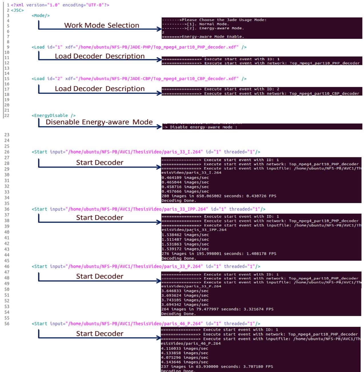
Figure 8-14 Verification on Reconfiguration Control Part 1
