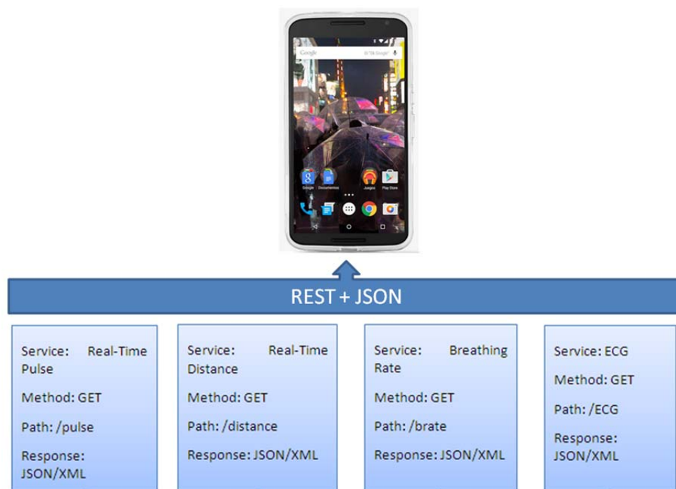
Figure 26 External interfaces for third party user applications (e.g.: a mobile application)
